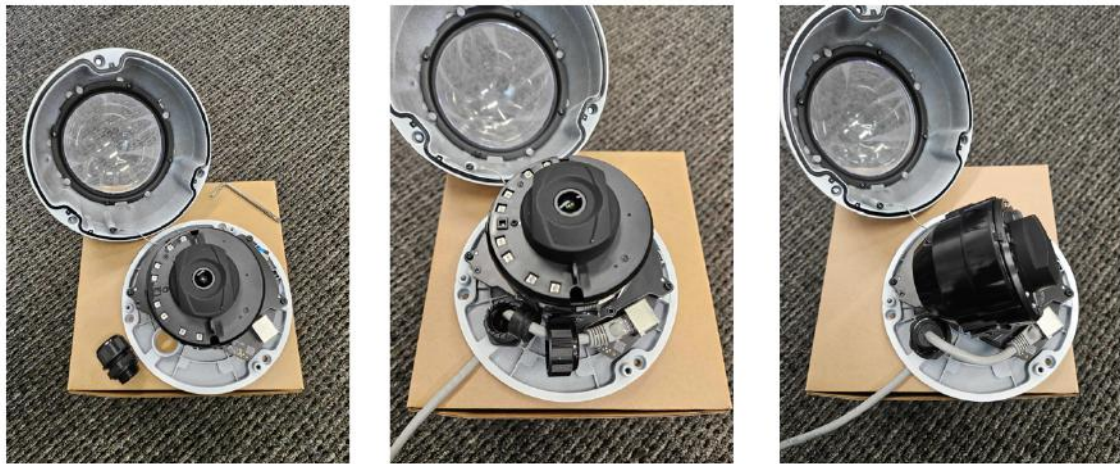
Figure 2: Installation of PoE cable
