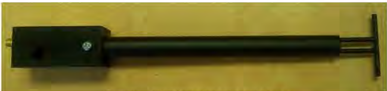
Figure 1 – MVG COMOSAR Validation Dipole
