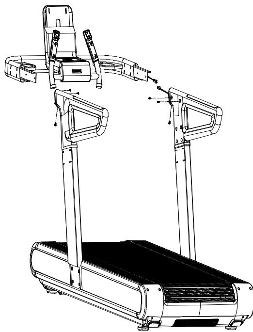
Step 4: take out the console from the packaging box, attach the console onto the console neck plate
