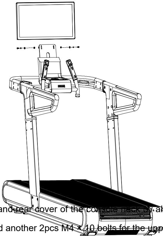
Step 5: As picture shown, fix front and rear cover of the ~~com~~ by aligning the holes, use 4pcs ST4 \* 16 screws for the bottom, and another 2pcs M4 \* 10 bolts for the upper. Then attach the upright cover to each upright by 4ea ST4 \* 16 screws.
