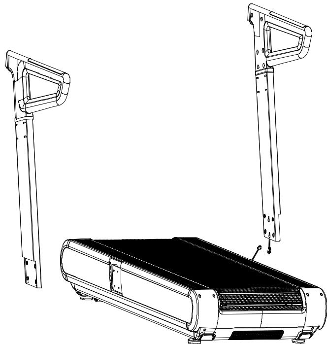
Step 3: As picture shown, connect the communication wire between console frame and handlebar, and tuck the excess wire into the handlebar. Insert the console frame clamp ring into the handlebar, align the hole and fix the inner side by 4ea M8 \* 20 bolts, tighten the bolts and cover the hole plug; Then fix the handlebar from the bottom by 2ea M8 \* 20 bolts. Tighten all upright bolts.
