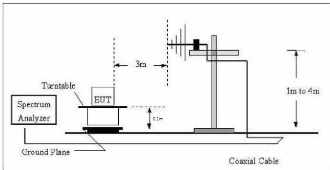
The test setup for emission measurement above 1 GHz
