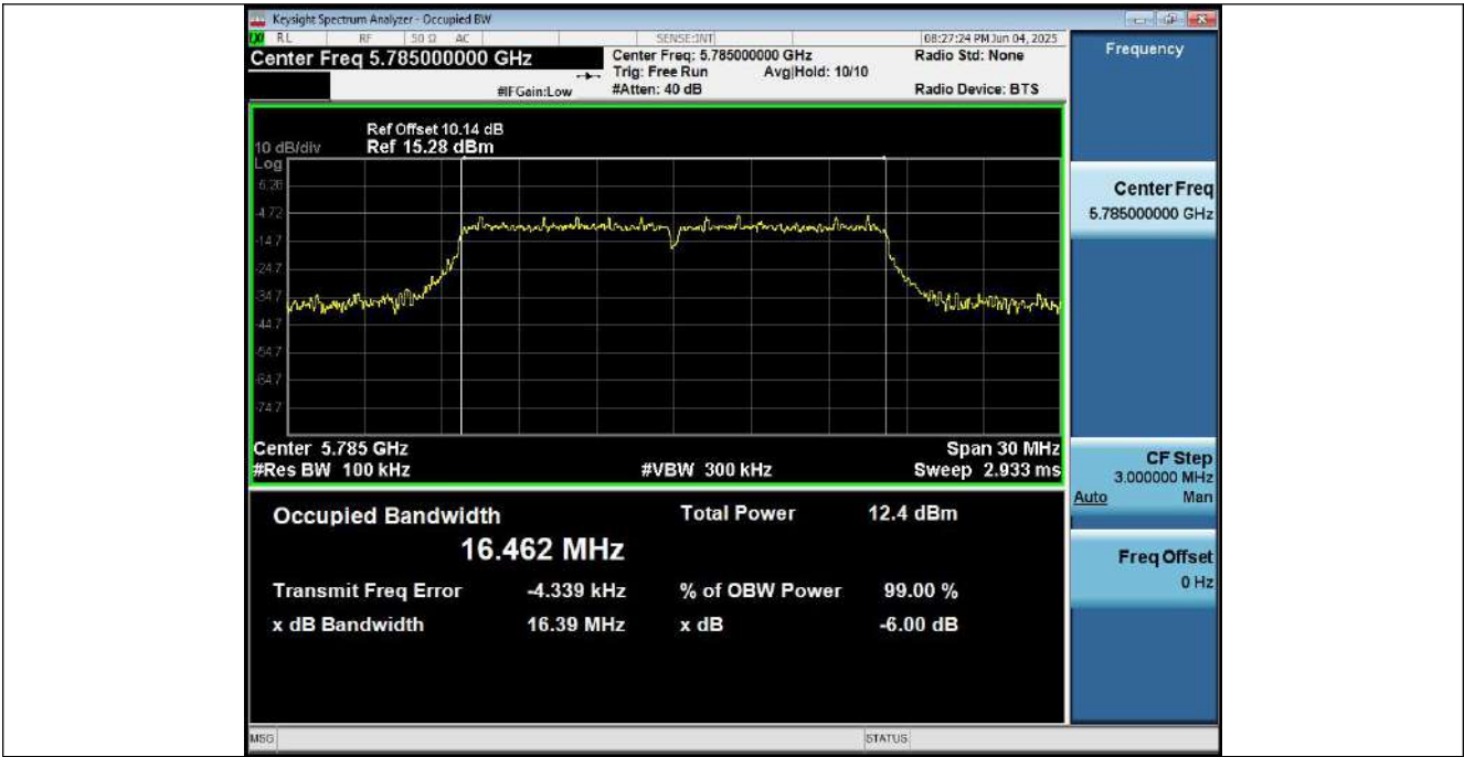
-6dB Emission Bandwidth NVNT ANT1 802 11a 5825 20M
