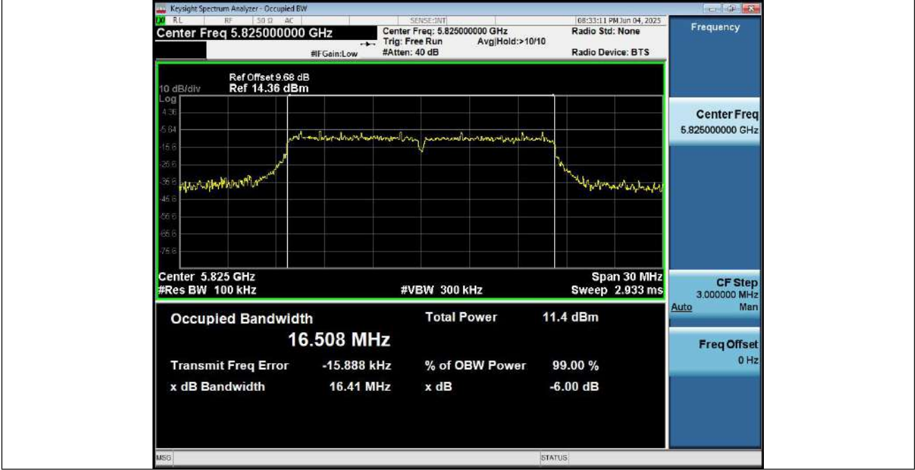
-6dB Emission Bandwidth NVNT ANT1 802 11a 5825 20M
