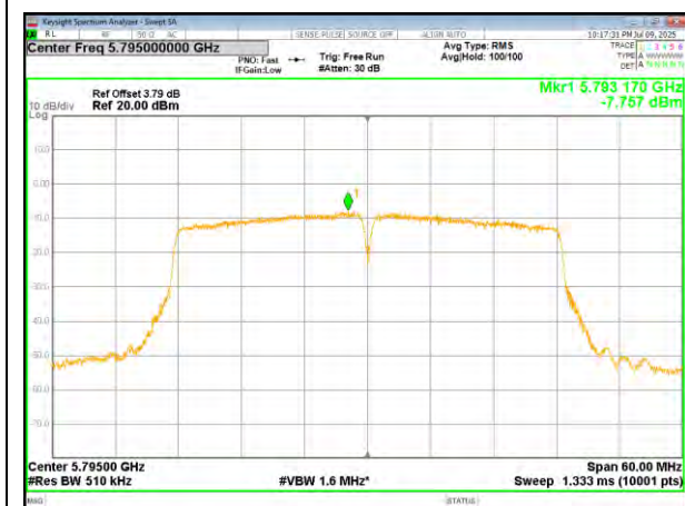
(802.11ac40) PSD plot on channel 159
