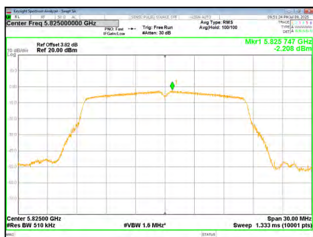
(802.11a) PSD plot on channel 165
