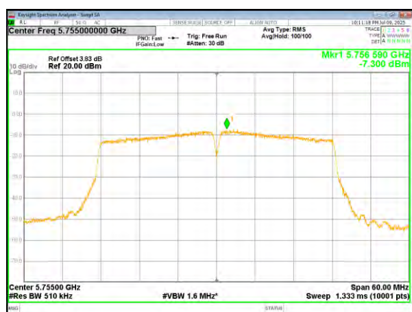
(802.11n40) PSD plot on channel 151
