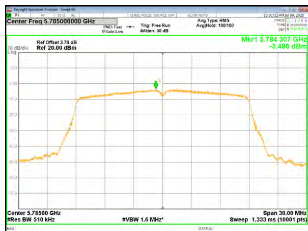
(802.11ac20) PSD plot on channel 165
