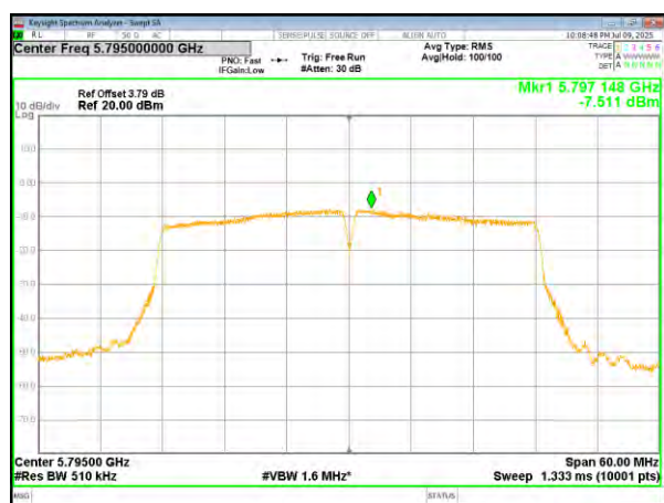
(802.11ac40) PSD plot on channel 151
