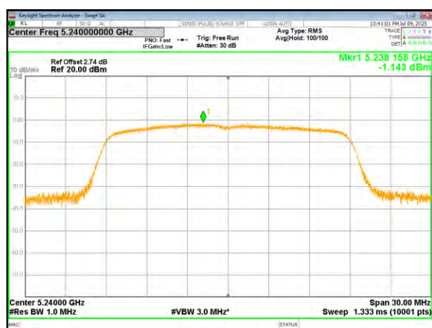
(802.11n20) PSD plot on channel 48
