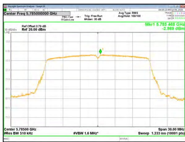
(802.11n20) PSD plot on channel 165
