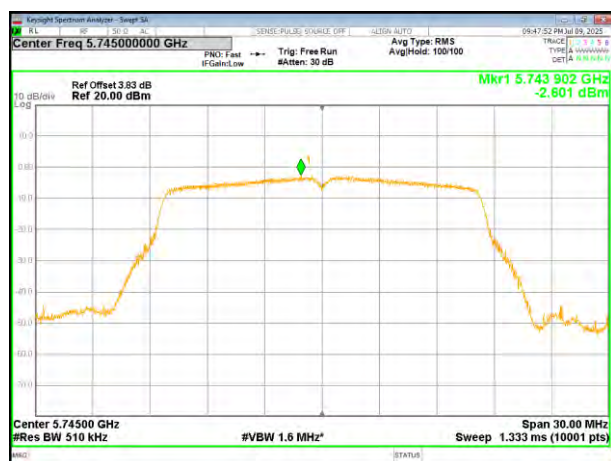
(802.11a) PSD plot on channel 157
