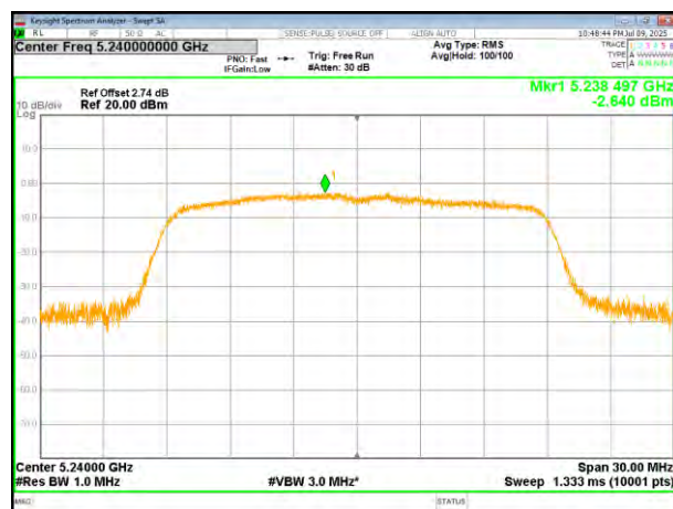
(802.11ac20) PSD plot on channel 48
