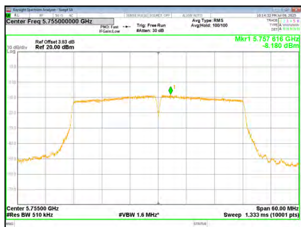
(802.11ac40) PSD plot on channel 151
