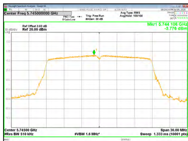
(802.11ac20) PSD plot on channel 149
