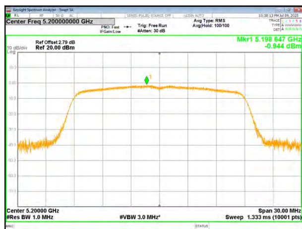
(802.11n20) PSD plot on channel 48
