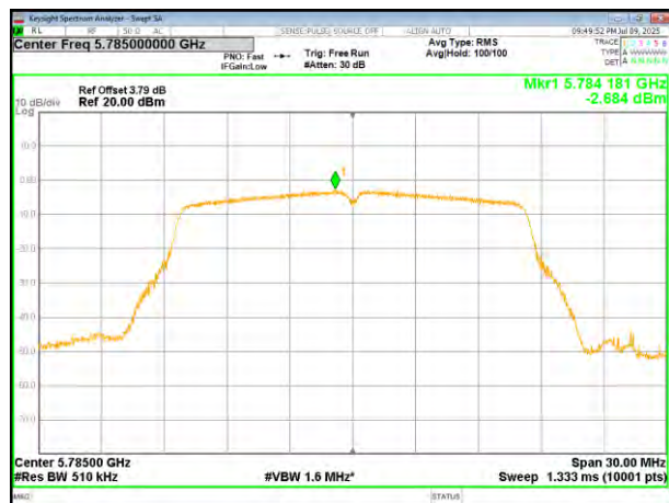
(802.11a) PSD plot on channel 165
