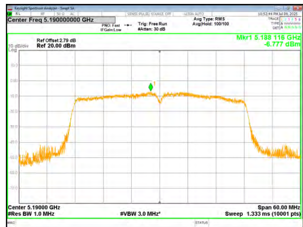
(802.11n40) PSD plot on channel 46
