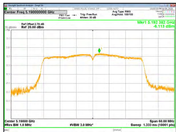
(802.11ac40) PSD plot on channel 38
