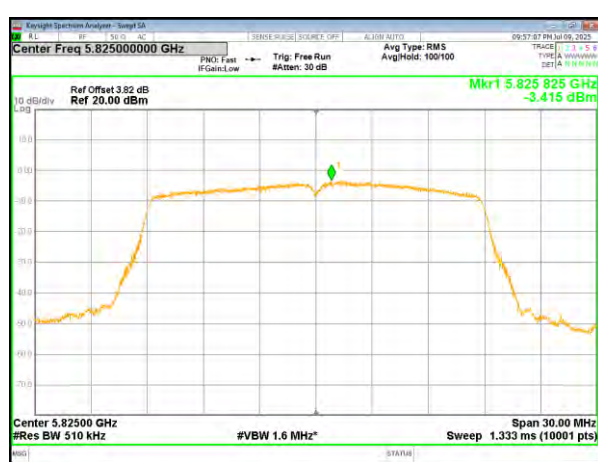
(802.11n20) PSD plot on channel 165
