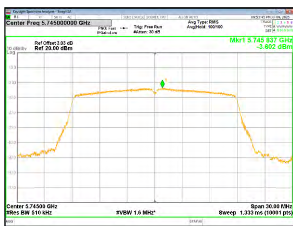
(802.11n20) PSD plot on channel 157
