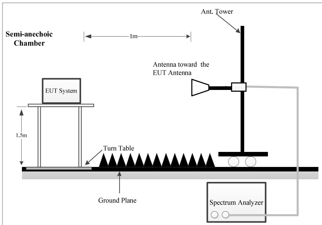
Place the measurement antenna at a measurement distance that is in the far-field of the measurement antenna, in the far-field of the EUT antenna. The EIRP test was performed at 1m distance, which was larger than the minimum test distance, please refer to section 4.2.4 for more detail.
