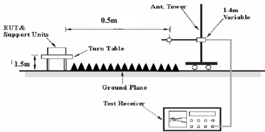
The radiated emission tests were performed in the 3 meters chamber test site, using the setup accordance with the ANSI C63.26-2015. The specification used was the FCC 95.3379 limits.
