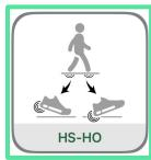
HS-HO Feedback: In this mode, vibrational feedback is given at each heel off and at each heel strike in the form of a vibration pulse.
