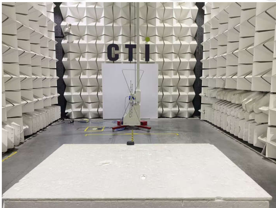
Radiated spurious emission Test Setup-1(Below 1GHz)
