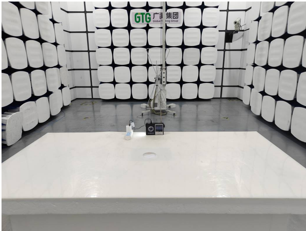
Radiated Measurement Photo
