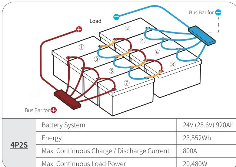
① As **-** of ① / ③ / ⑤ / ⑦ is connected in series with **+** of ② / ④ / ⑥ / ⑧, please do not connect **-** of ① / ③ / ⑤ / ⑦ with **-** of load or **+** of ② / ④ / ⑥ / ⑧ with **+** of load, otherwise the battery system will fail to connect in series.
