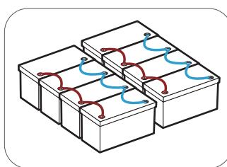
Connect the batteries in parallel.
