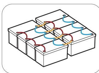
Connect the paralleled battery systems in series.
