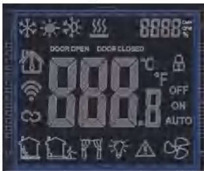
(W) Version 2 8918Q Thermostat panel Fig.22
