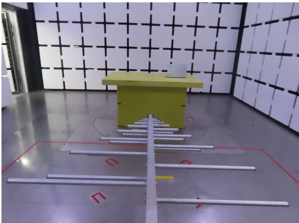
**Radiated Emissions Test Photos****Harmonic 1 GHz - 18GHz & Band edge**
