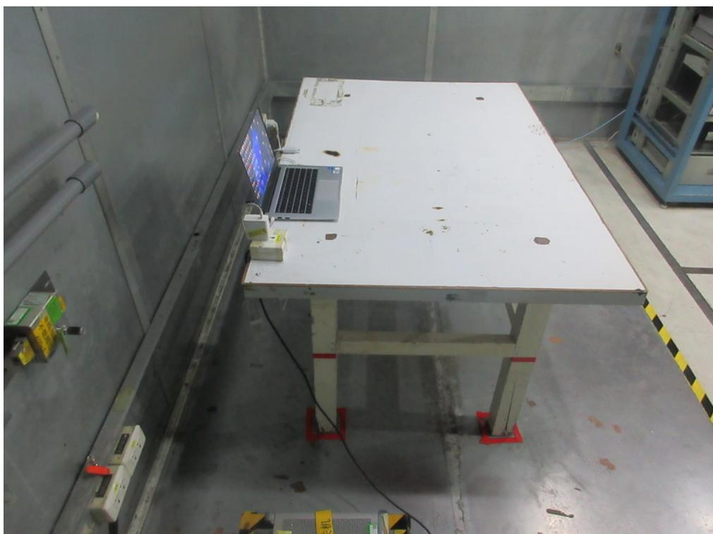
**Radiated Emissions Test Photos****9 kHz to 30 MHz**
