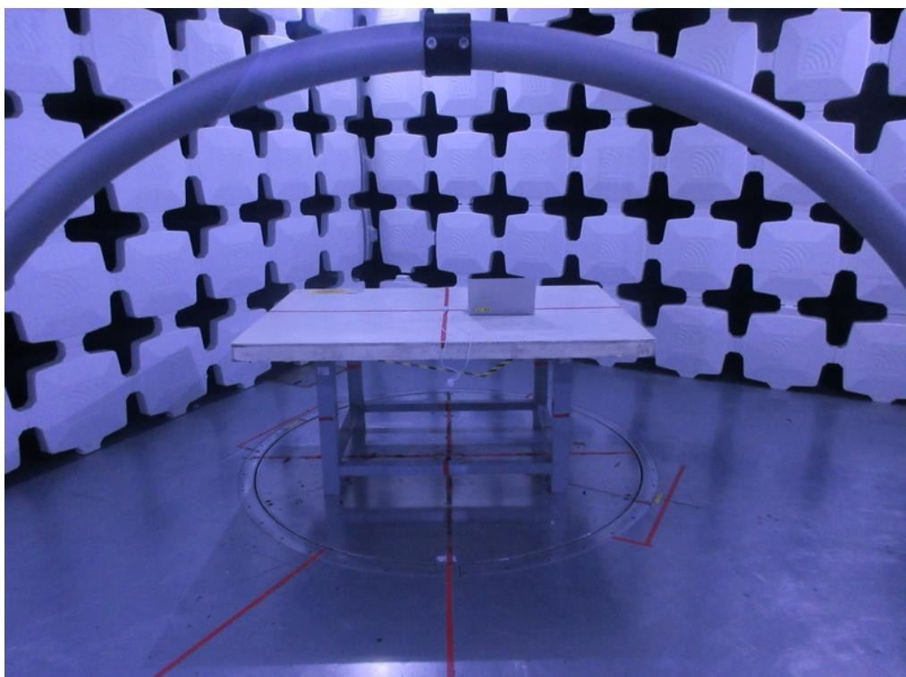
**Radiated Emissions Test Photos****30 MHz to 1000 MHz**
