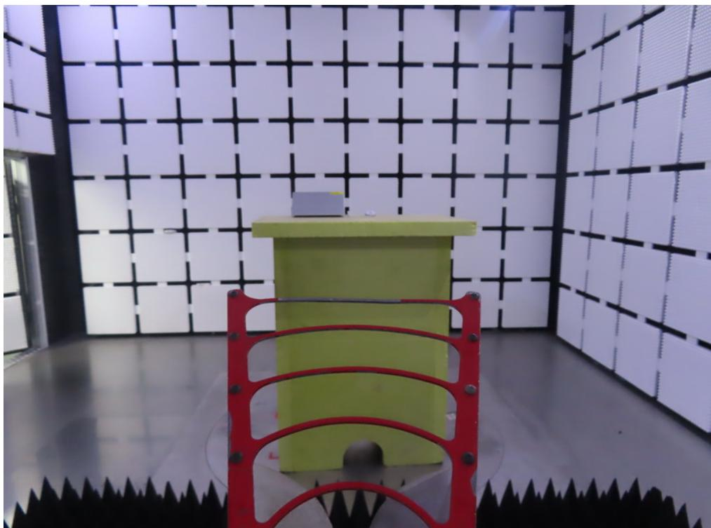
**Radiated Emissions Test Photos****Harmonic Above 18GHz**
