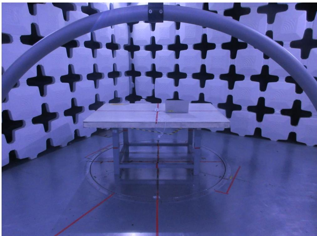
**Radiated Emissions Test Photos****30 MHz to 1000 MHz**
