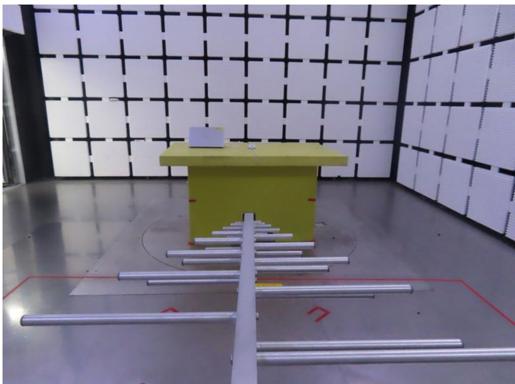
**Radiated Emissions Test Photos****Harmonic 1 GHz - 18GHz & Band edge**
