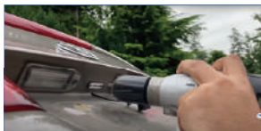
J.Apply the 3M adhesive to the rear camera bracket, and adjust the angle.
