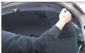
G.Remove the trunk panel.
