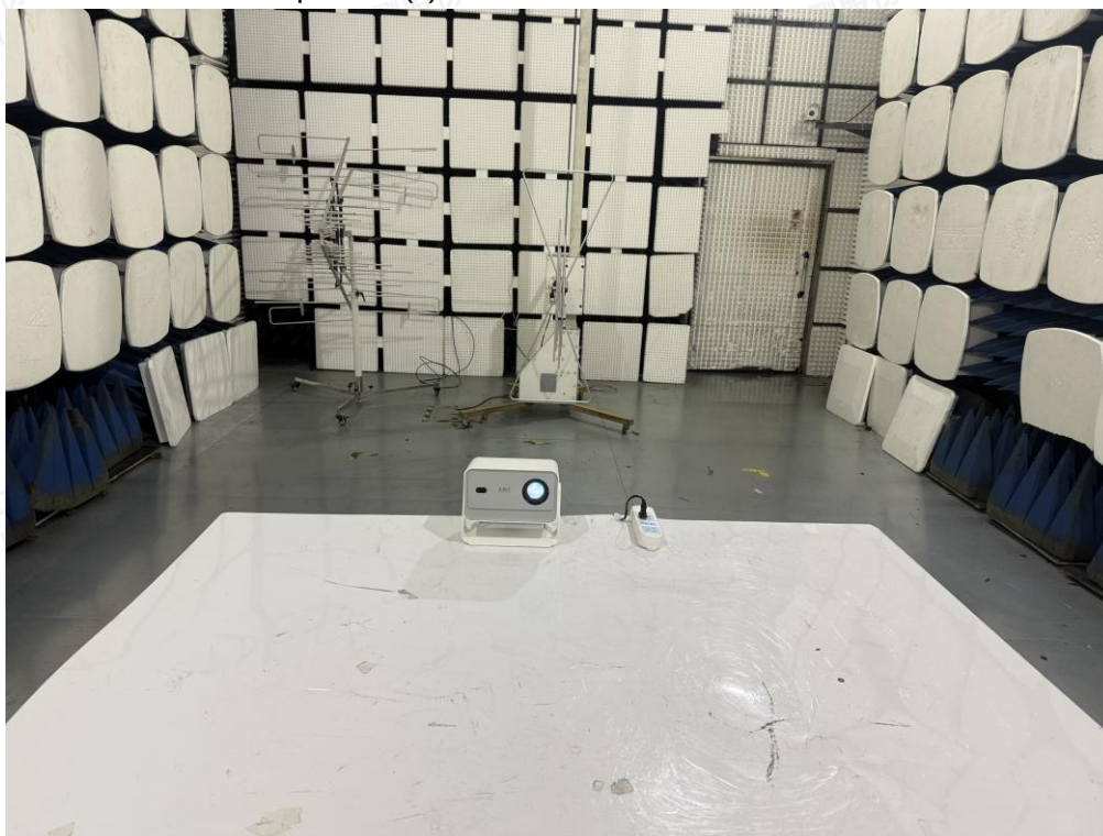
Test Setup Photo(s) of Radiated Emissions Measurement
