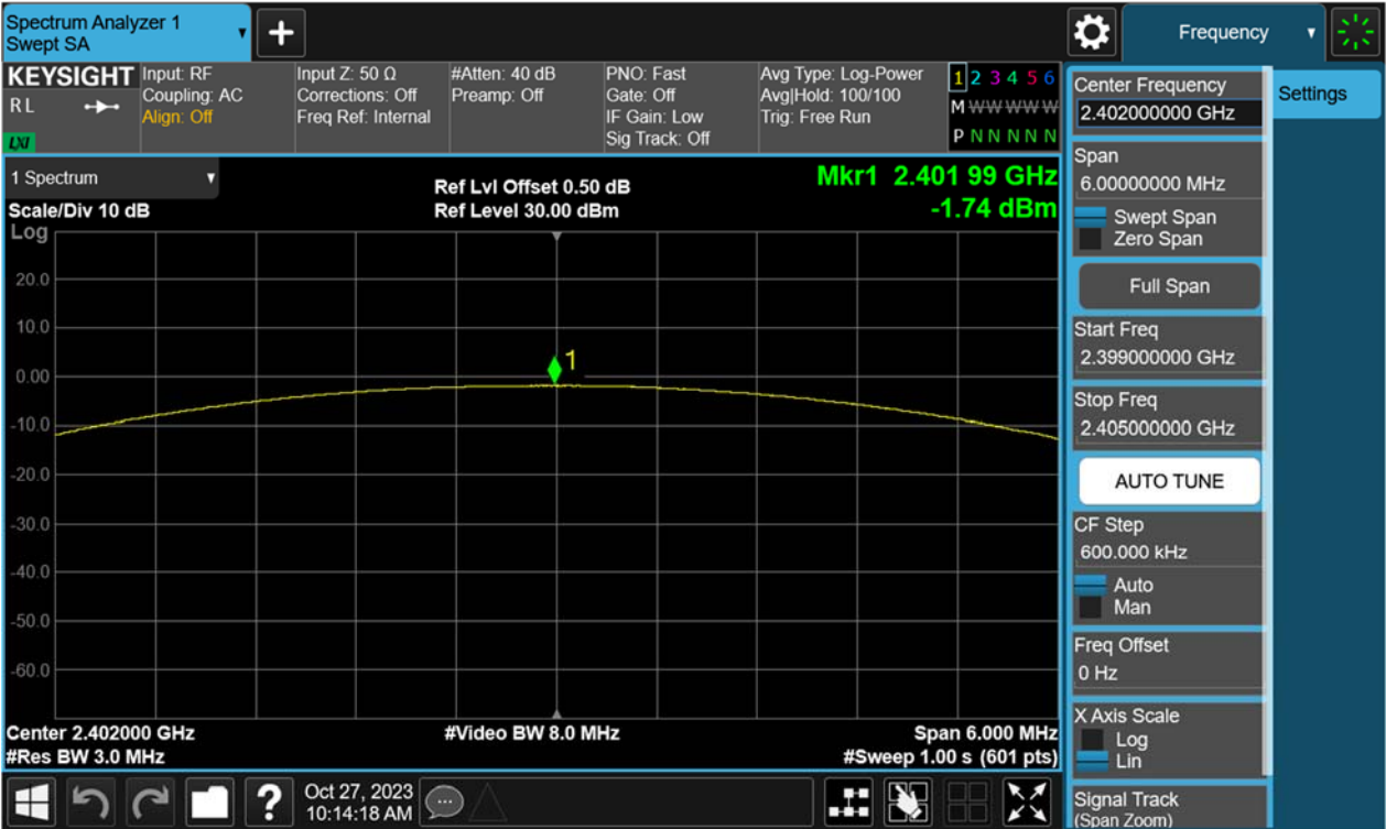
Figure 4: Maximum Peak Output Power, 2402MHz, \pi/4 -DQPSK
