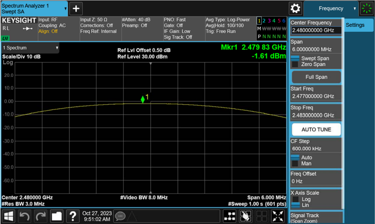
Figure 4: Maximum Peak Output Power, 2402MHz, \pi/4 -DQPSK
