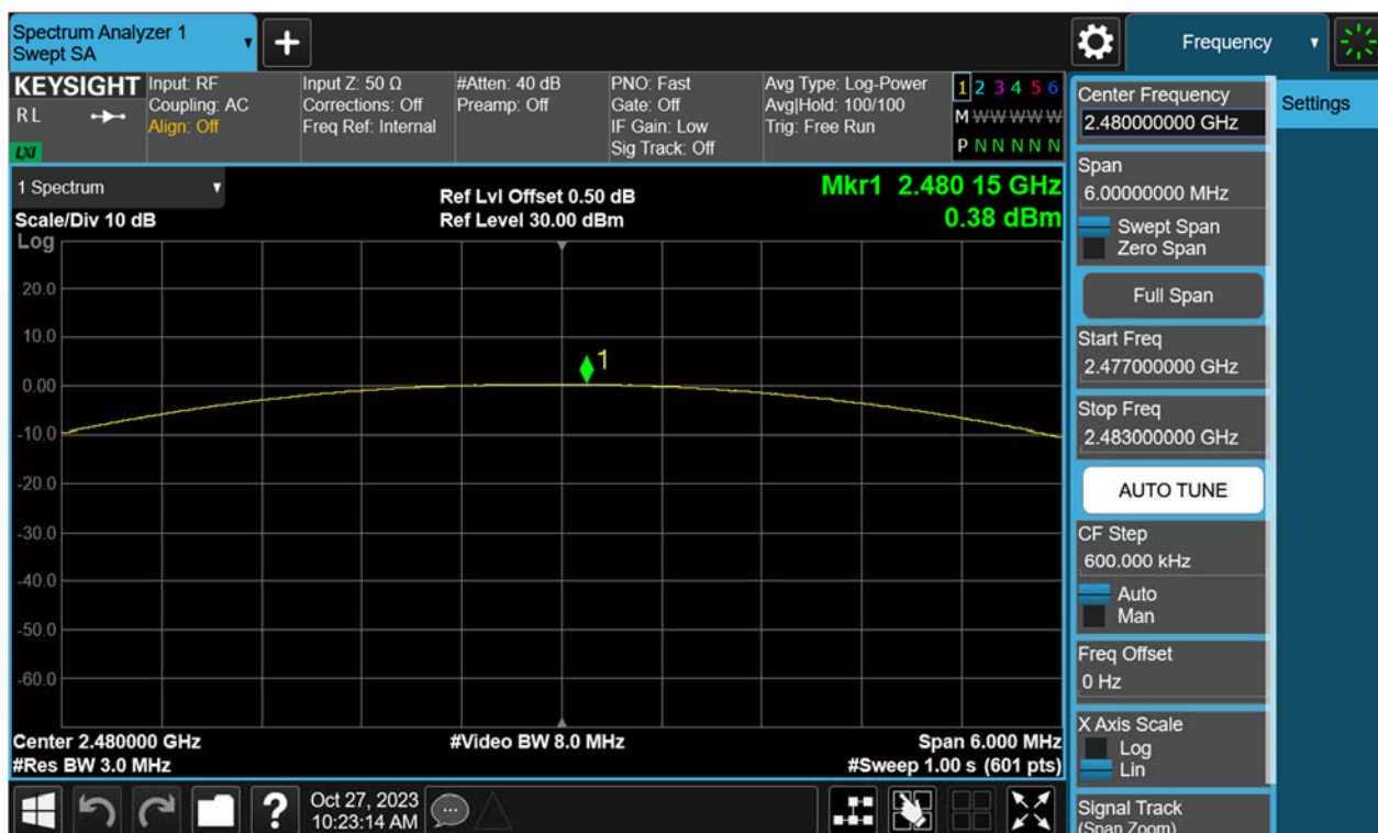
Figure 6: Maximum Peak Output Power, 2480MHz, \pi/4 -DQPSK
