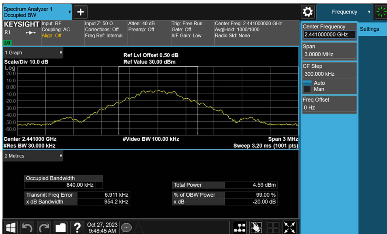
Figure 11: 20dB Bandwidth and 99% Bandwidth, 2441MHz, GFSK
