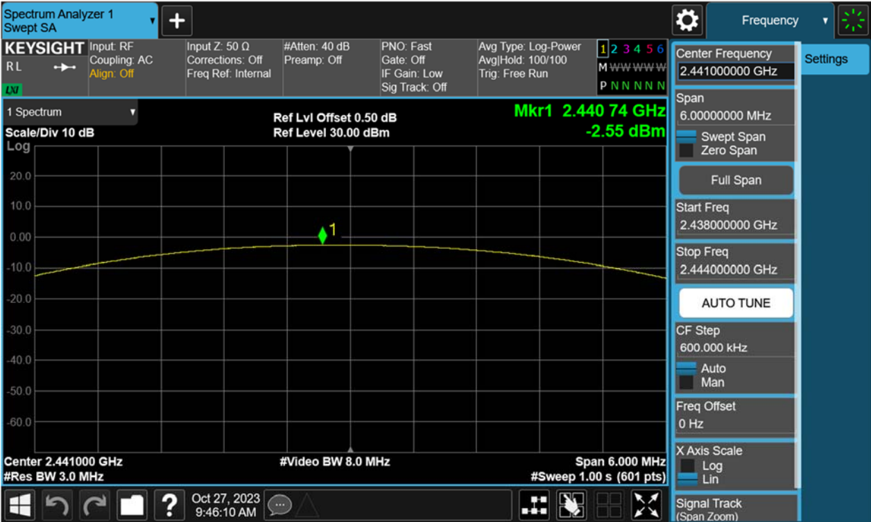
Figure 2: Maximum Peak Output Power, 2441MHz, GFSK
