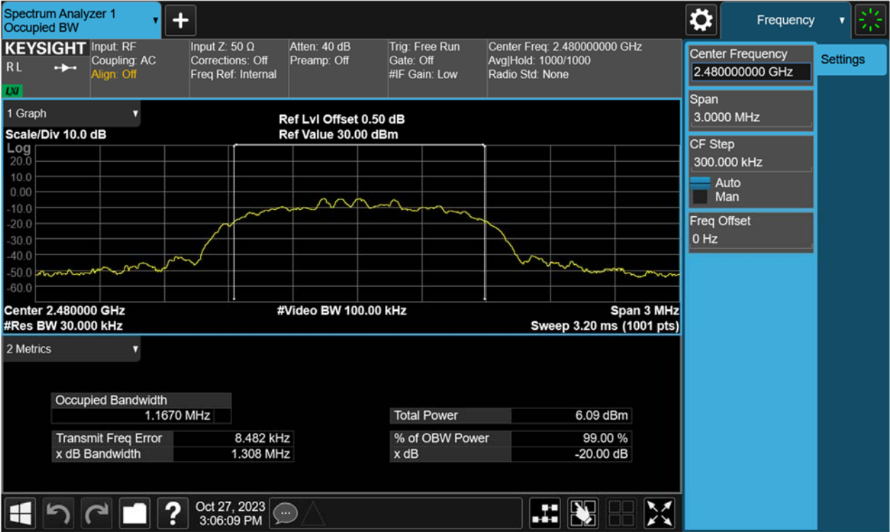
Figure 18: 20dB Bandwidth and 99% Bandwidth, 2480MHz, 8-DPSK
