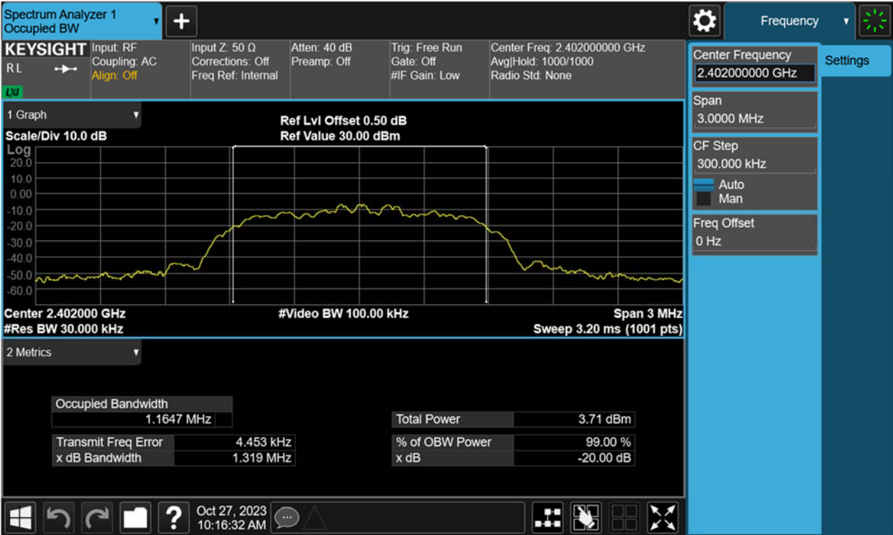
Figure 13: 20dB Bandwidth and 99% Bandwidth, 2402MHz, \pi /4-DQPSK
