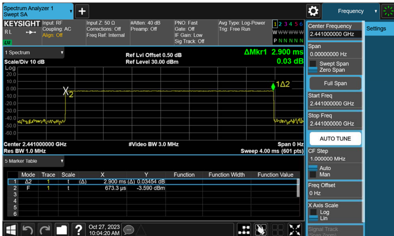
Figure 40: Time of Occupancy, 2441MHz, \pi/4 -DQPSK DH1
