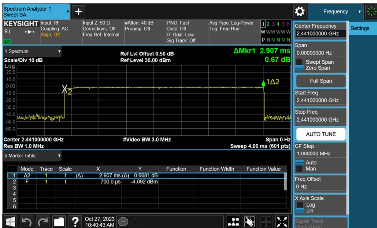
Figure 42: Time of Occupancy, 2441MHz, \pi/4 -DQPSK DH5
