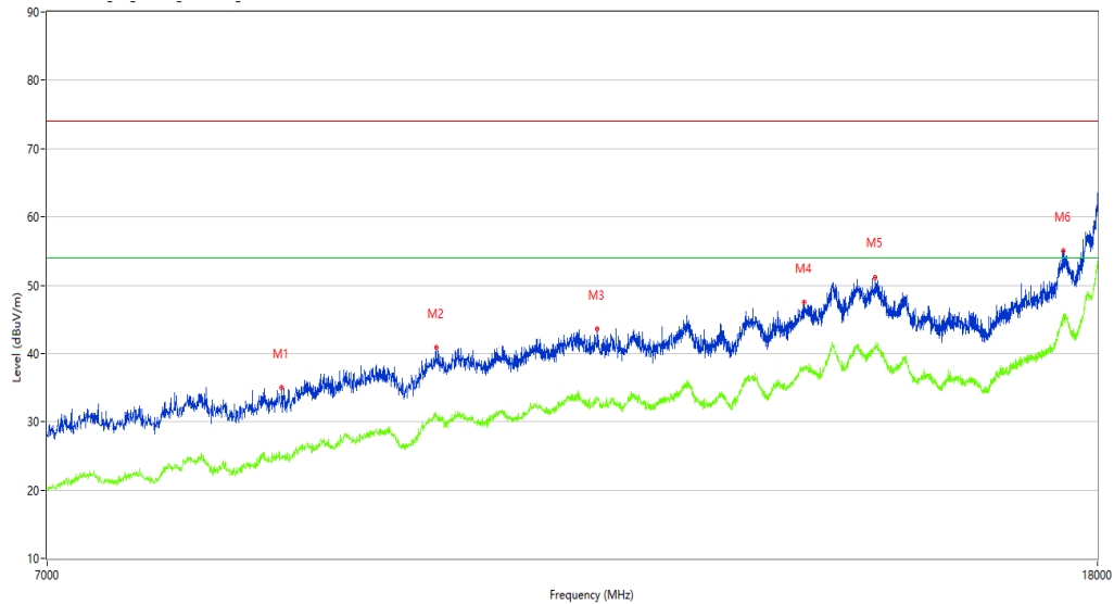
R Emission Test case_FCC_Part 15C_FCC 15.247_7GHz-18GHz
