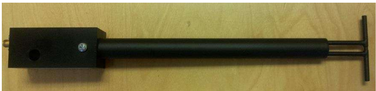
Figure 1 – MVG COMOSAR Validation Dipole
