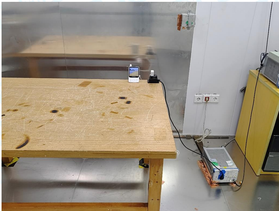
Photo of Setup for Conducted Emission
