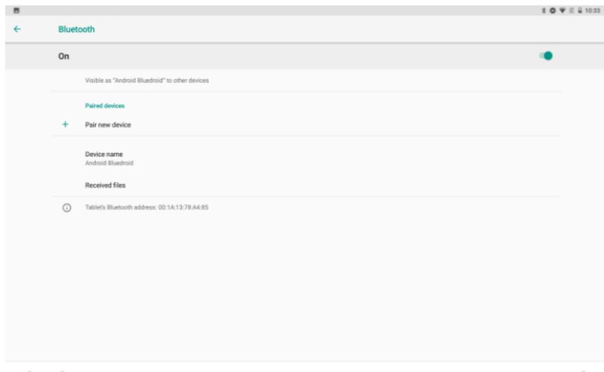
Touch the desired Bluetooth device to start pairing. Then according to the indications on both sides, users can complete the connection successfully in seconds. After pairing, you can share files between the unit and the Bluetooth device.
