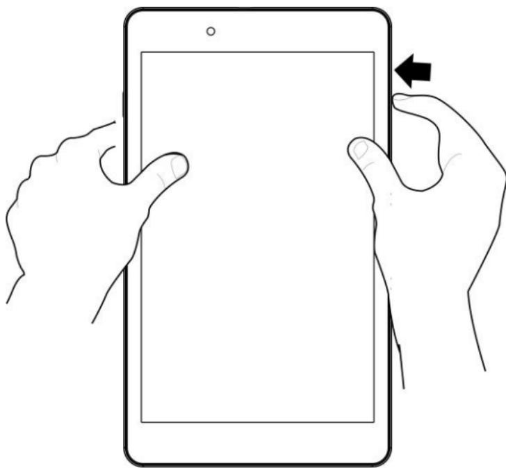
Press the power button once to access standby mode and press again to wake it up;
