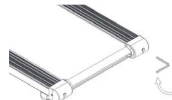
3. If the running belt leans to the right, rotate the right adjusting bolt clockwise by 1/4 turn and pause for 30 seconds, then the running belt automatically returns to normal. If it does not return to normal, please repeat the above method for adjustment.
