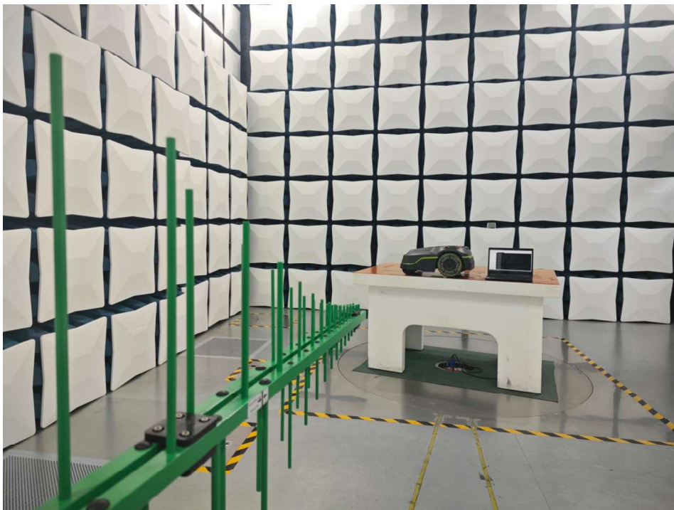
Test Set-up: Radiated spurious emission Below 1GHz
