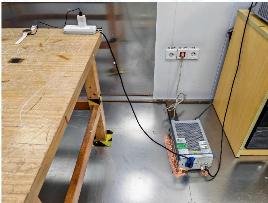
Photo of Setup for Radiated Emission (30MHz~1GHz)
