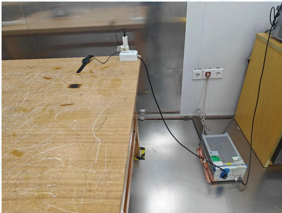
Photo of Setup for Conducted Emission
