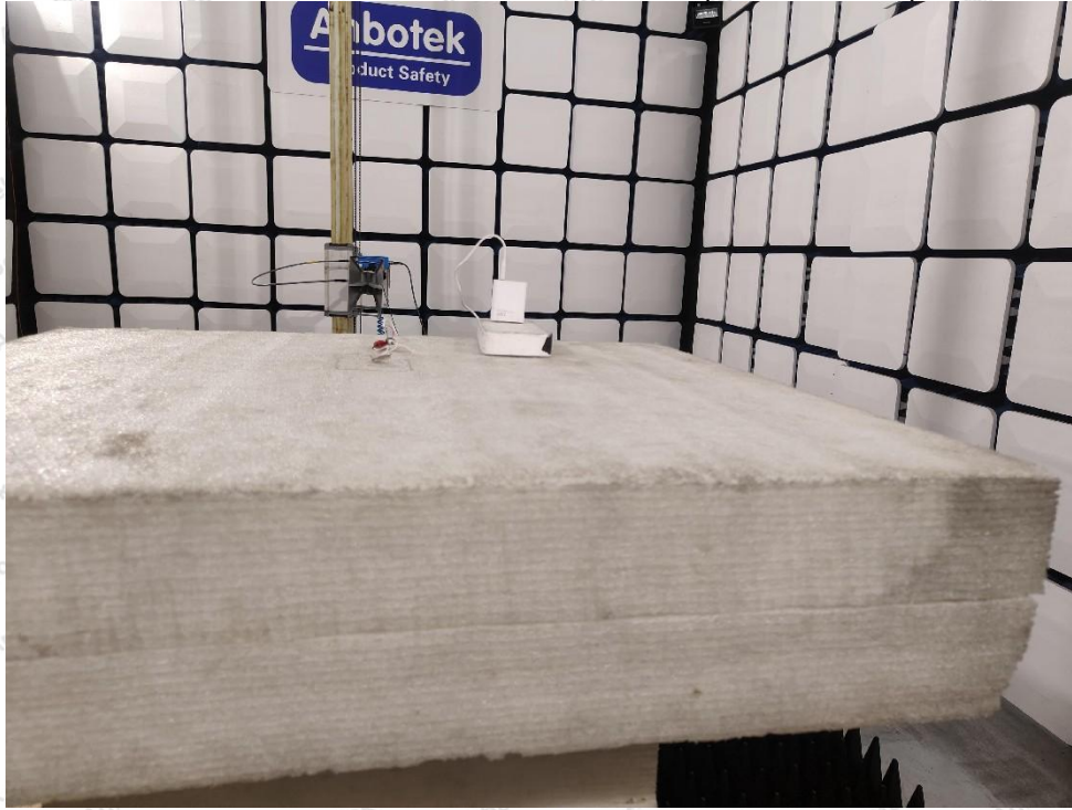
Photo of Radiation Emission Test (above 1GHz)
