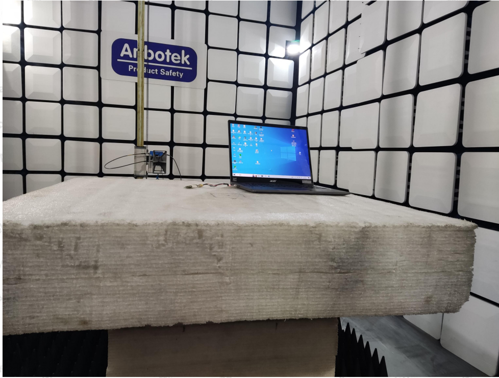
Photo of Radiation Emission Test (above 1GHz)
