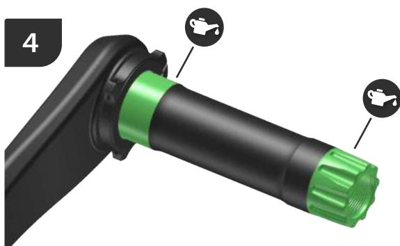
Lightly grease the bearing contact surfaces on the spindle and the bottom bracket.
