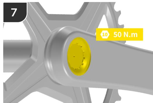
Tighten the drive side crank by using a 10 mm hex wrench (50Nm).
