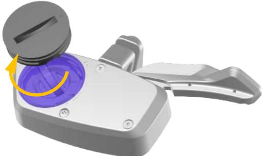
Insert a new CR2032 battery with the positive + sign facing into the cover.
