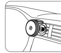
2. Insert the hook into the car air outlet vane and tighten to lock. when you hear 'clatter' sounds, it means the mount has been fixed tightly.
