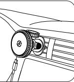
3. Connect the charging cable to the charging interface.
