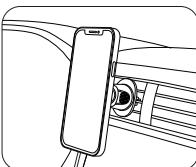
4. Put the phone on the magnet head, adjust the best viewing angle.
