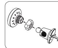
1. Insert the adjuster into ball joint of air vent mount, insert the ball into the socket at the back of magnet head, turn the adjuster to tighten.
