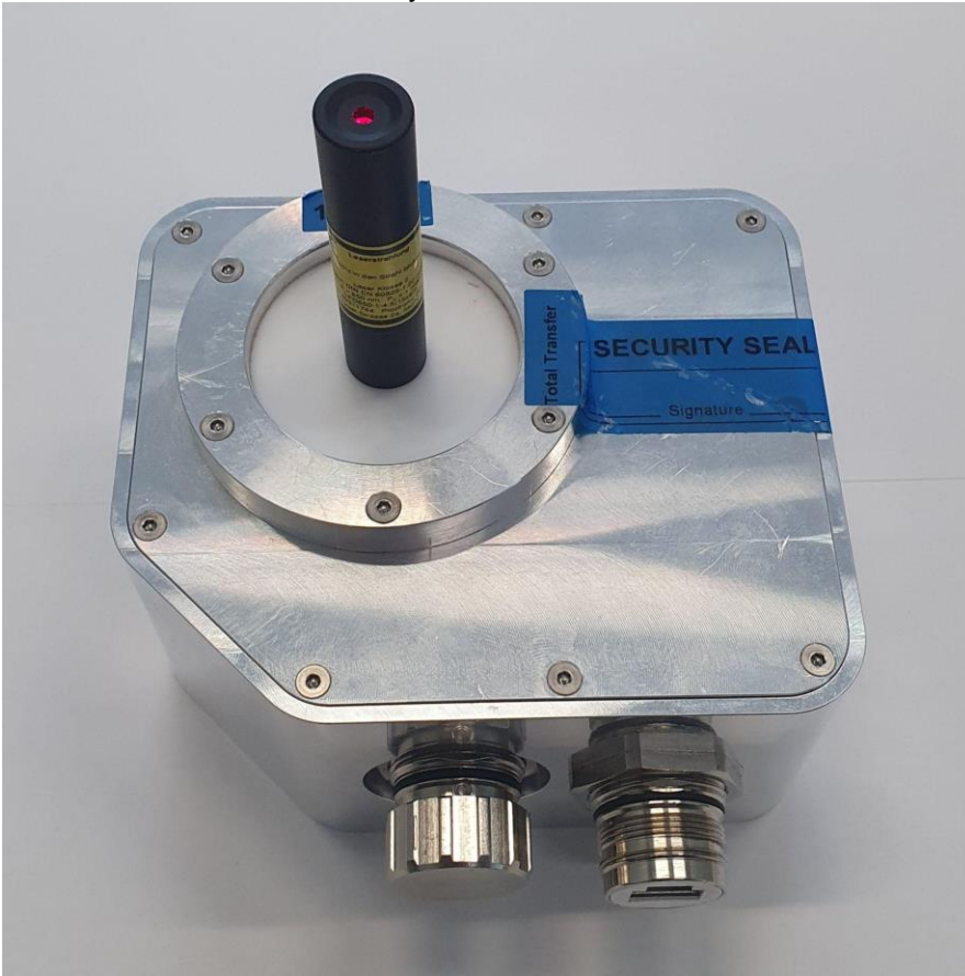
Figure: The alignment laser is positioned centrally on the cover plate of the sensor unit
