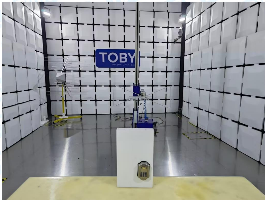
Photo of Setup for Radiated Emission (30MHz~1GHz)
