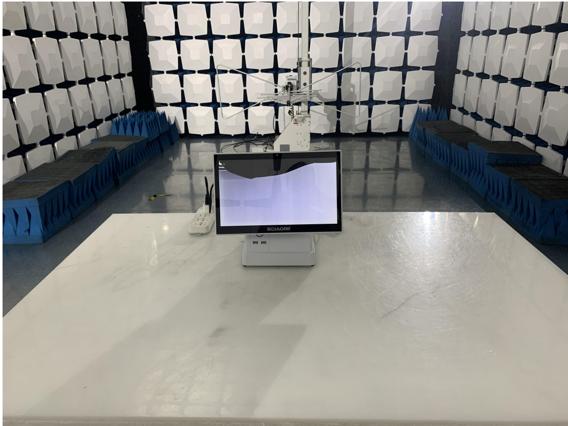
Blow 1GHz for radiated emission test setup
