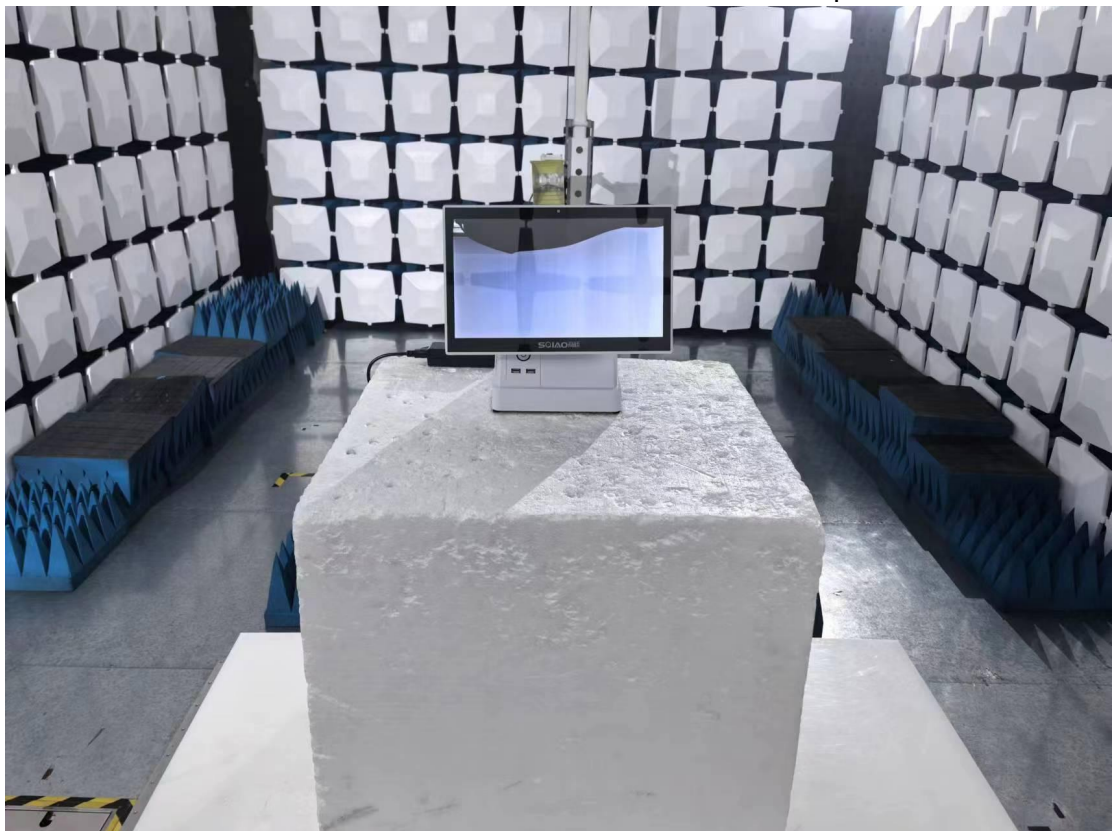
Above 1GHz for radiated emission test setup
