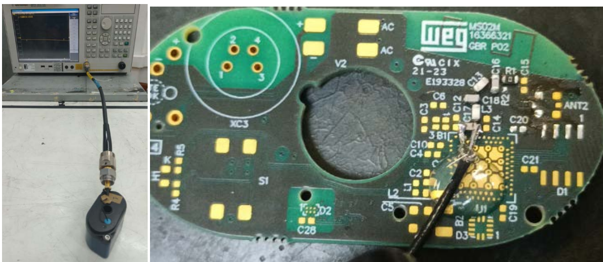
Figure 3- Product set up for Return Loss Measurement.
