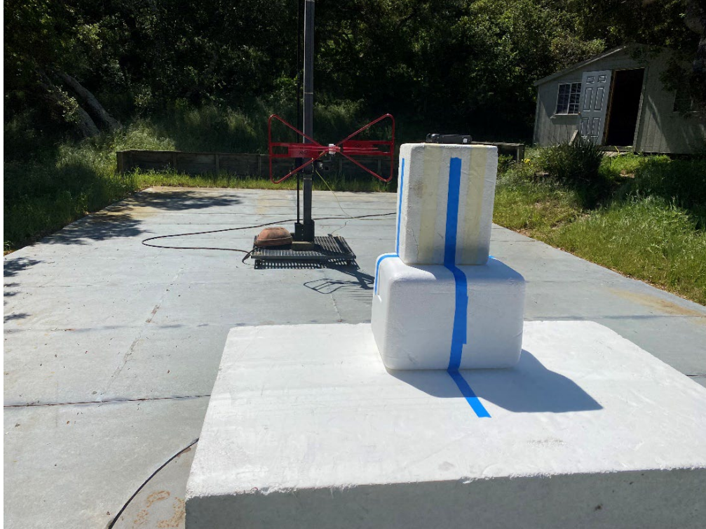
30 MHz – 1 GHz Test Setup
