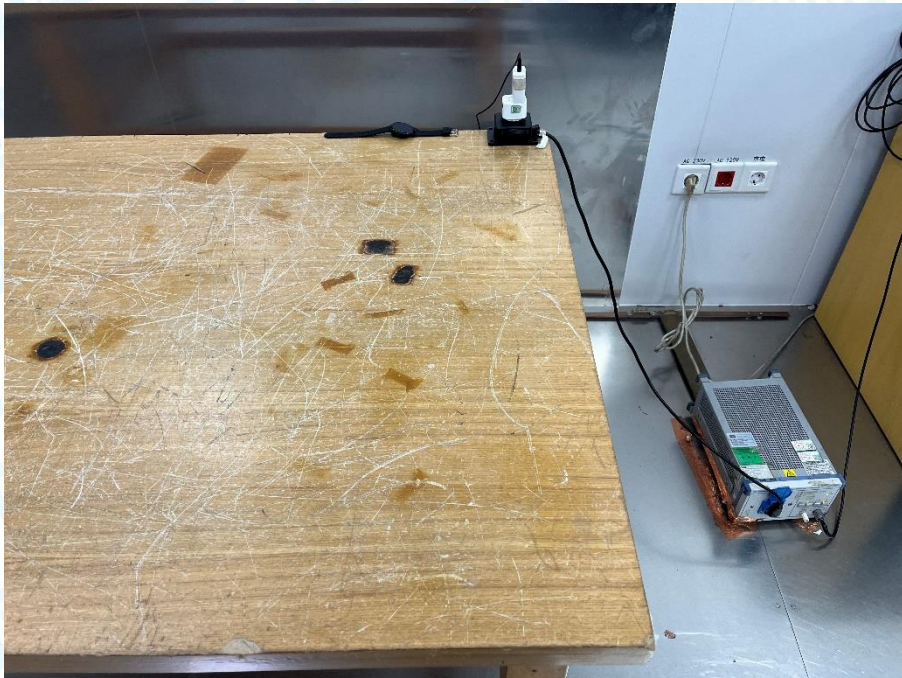
Photo of Setup for Radiated Emission (30MHz~1GHz)
