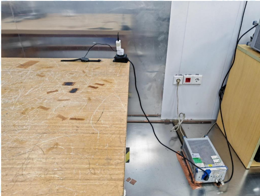
Photo of Setup for Conducted Emission(AC POWER)
