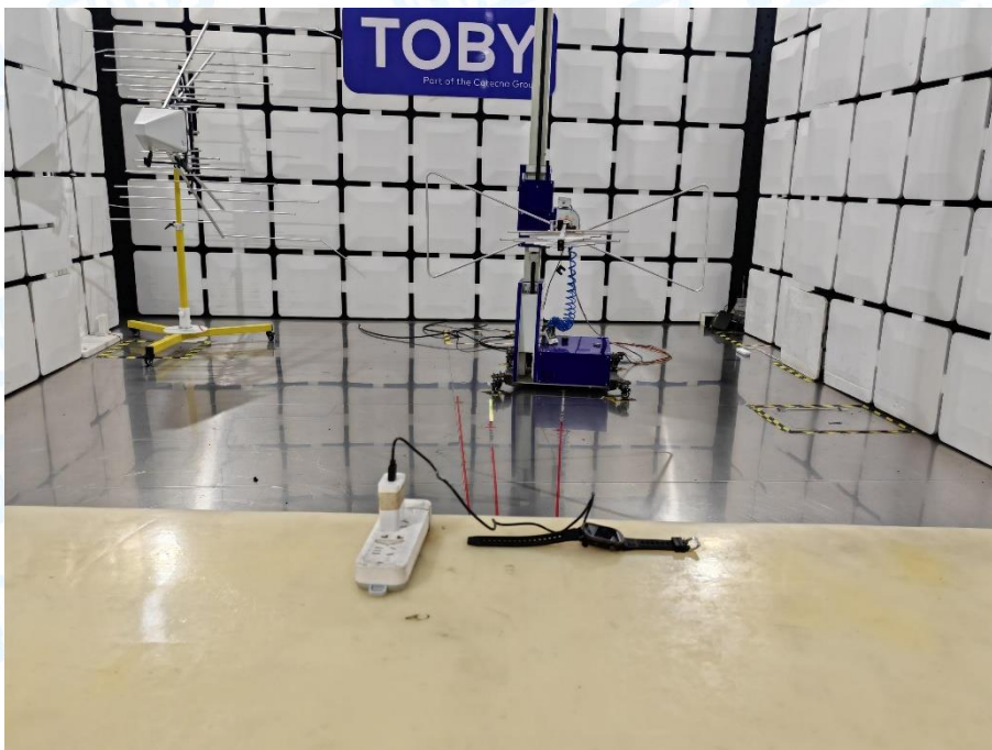
Photo of Setup for Radiated Emission (30MHz~1GHz)
