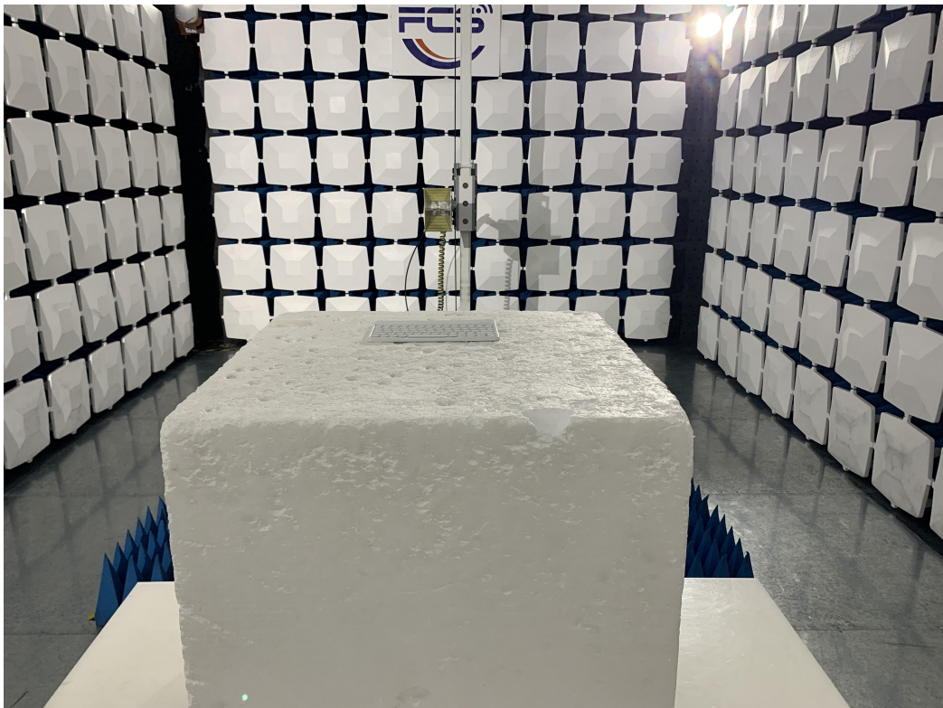
Above 1GHz for radiated emission test setup
