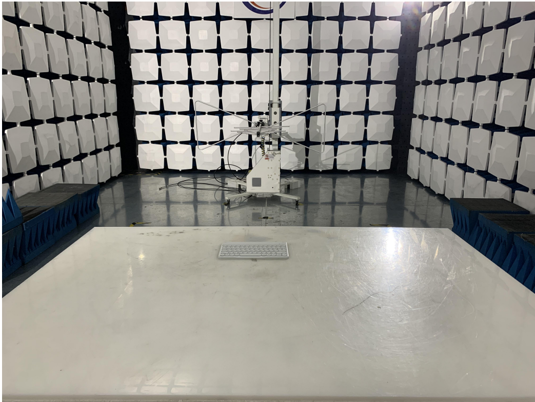
Above 1GHz for radiated emission test setup
