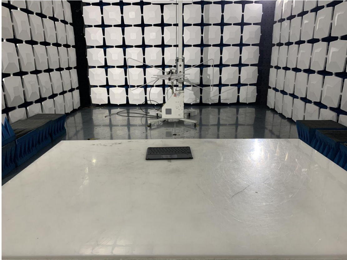
Above 1GHz for radiated emission test setup
