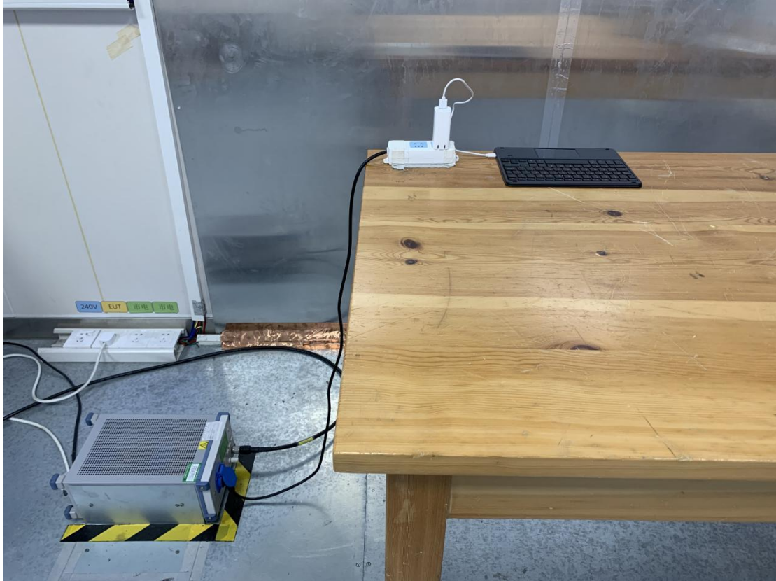
Conducted emission test setup
