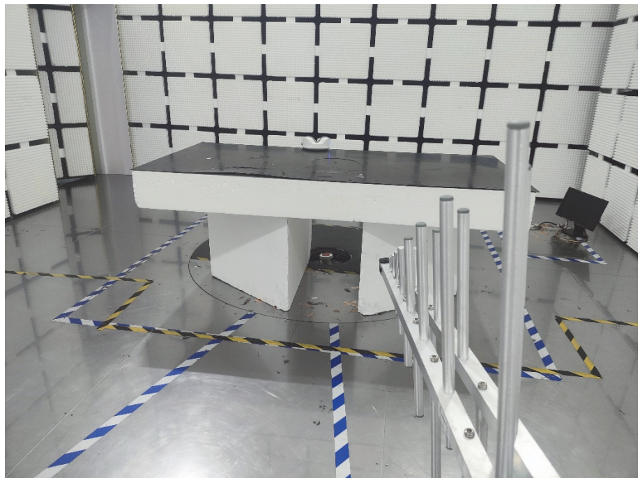
Radiation Emission Test Setup (30MHz to 1GHz)
