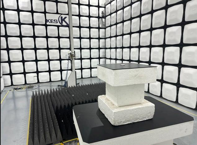
A photograph of an anechoic chamber. The walls are covered in white, rectangular acoustic absorption panels. The floor is black with a white checkered pattern. In the center, there is a white rectangular object on a white pedestal, and a blue and yellow tripod-mounted device. The KESK logo is visible on the left wall.                          | N/A               |
