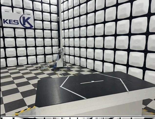
A photograph of an anechoic chamber, similar to the one above. The walls are covered in white, rectangular acoustic absorption panels. The floor is black with a white checkered pattern. In the center, there is a white rectangular object on a white pedestal, and a blue and yellow tripod-mounted device. The KESK logo is visible on the left wall. | N/A               |
