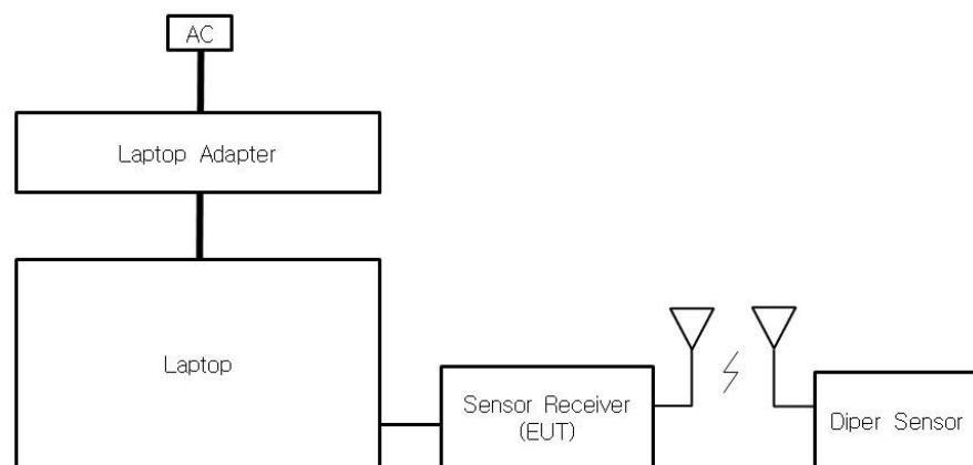
EUT -Diper Sensor : 902.5 MHz(Send/Receive)
