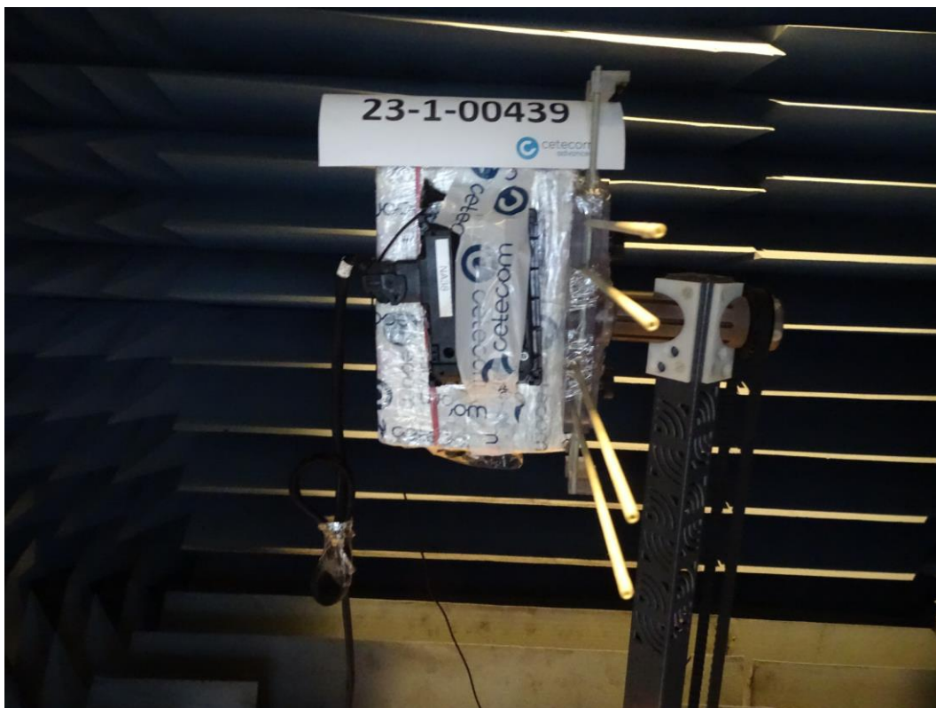
Fig. Mea.: 7 : Measurements in the fully anechoic chamber 2, close up view
