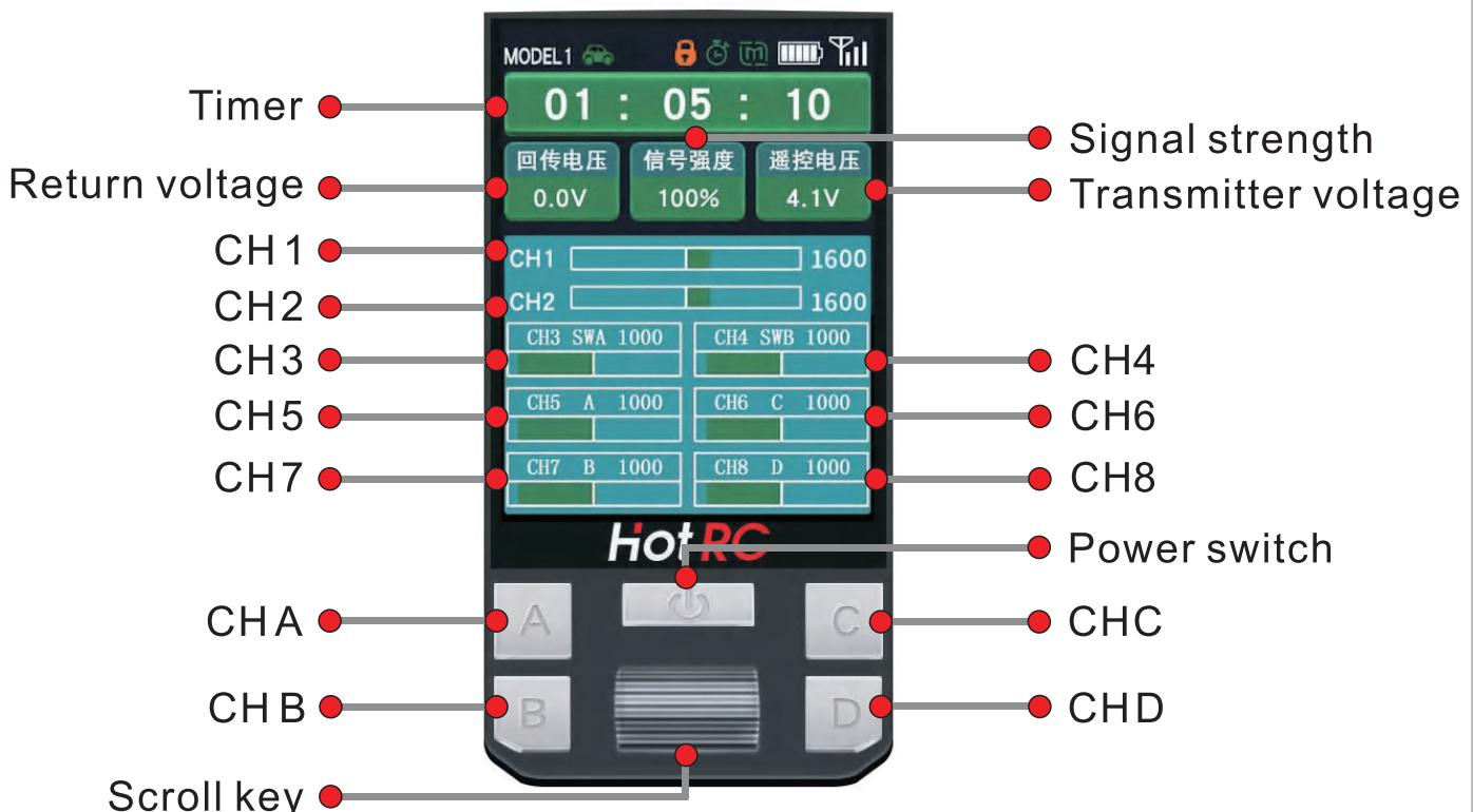
【Power switch】: long press to turn on and off, short press to return.
