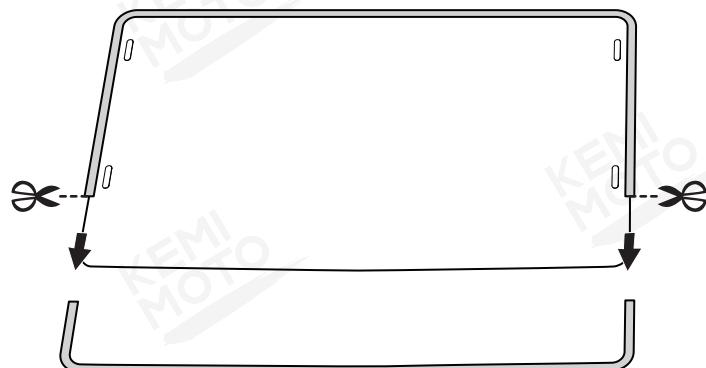
**5** Separate the sealing strip [2] and stick the LED strip [1] in the middle of the sealing strip [2], then tightly pinch the sealing strip [2] onto the windshield edge. (Please do not apply excessive force)
