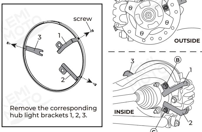
Remove the corresponding hub light brackets 1, 2, 3.
