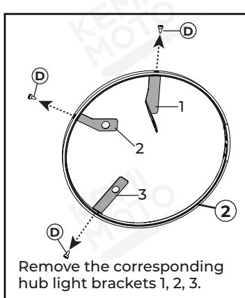
Remove the corresponding hub light brackets 1, 2, 3.
