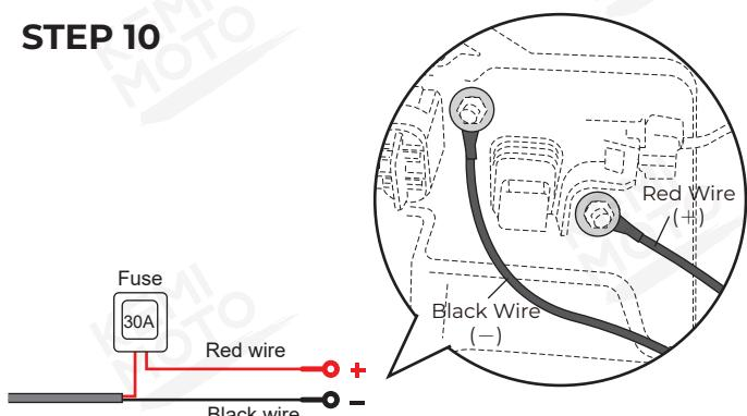
For power instructions: Lift the driver's seat, find the original car power supply, and connect the corresponding positive and negative terminals.
