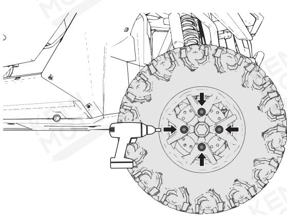
Finally reinstall the front right tire and tighten the screws.
