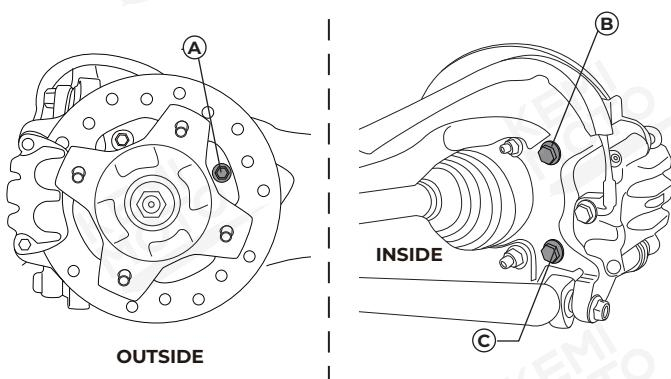
Loosen screw A to rotate out the height of the installation bracket, and remove screws B and C.
