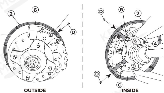
Insert the outer ring of the R-front hub light ② into the bracket, align the holes with the bracket holes, and lock the removed small hub light screws D back onto the bracket, then tighten screws A, B, and C.
