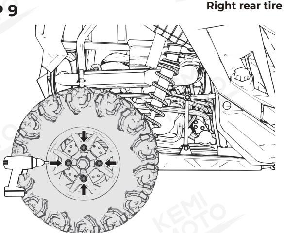
Finally reinstall the right rear tire and tighten the screws.
