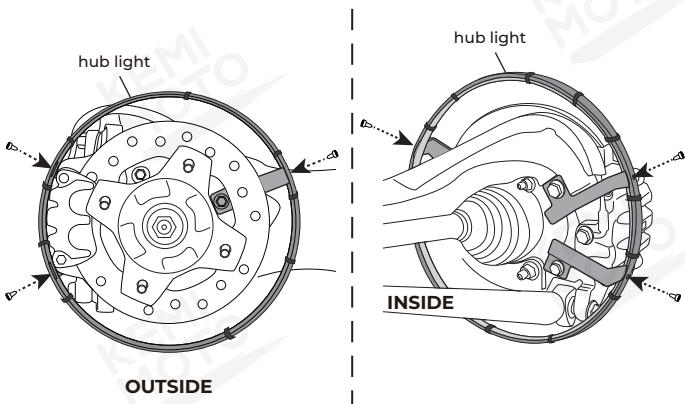
Insert the outer ring of the hub light into the bracket, align the holes with the bracket holes, and lock the removed small hub light screws back onto the bracket, then tighten screws A, B, and C.
