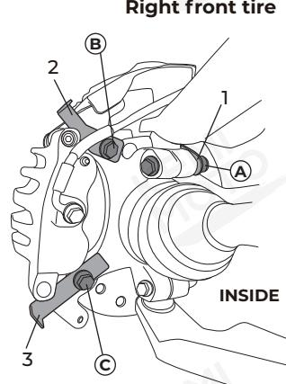
Insert them into the corresponding slots A-1, B-2, C-3 (pay attention to the direction of the bracket bending), slightly tighten screws A, B, and C just enough to clamp the bracket without fully tightening them.
