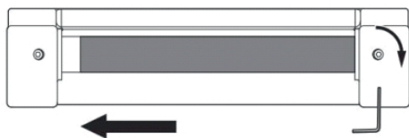
The running belt is leaning to the right, tighten the right
