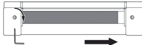
The running belt leans to the left, tighten the left
